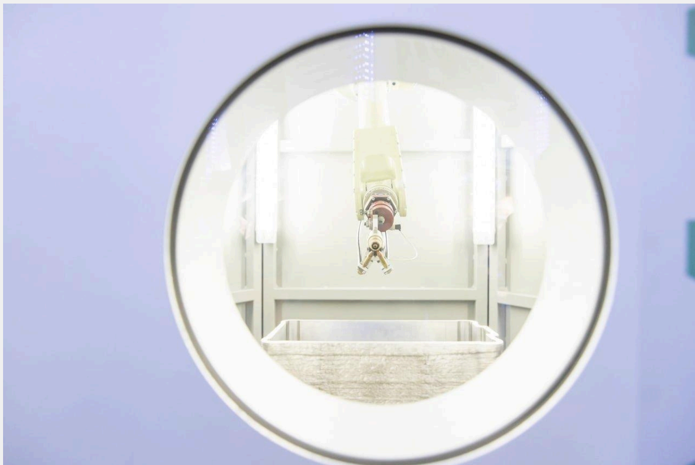
Welding robot inside the 'prism'. Image Credit: Oleg Panchenko
