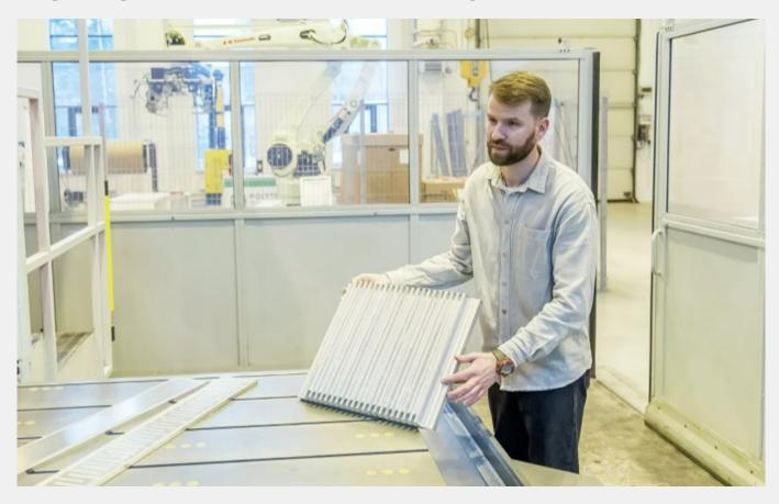
Researchers from Peter the Great St.Petersburg Polytechnic University (SPbPU) invented a durable and compact radiator for lithium-ion batteries, which in the future can be used for electric vehicles. The radiator was developed using friction stir welding technology.
